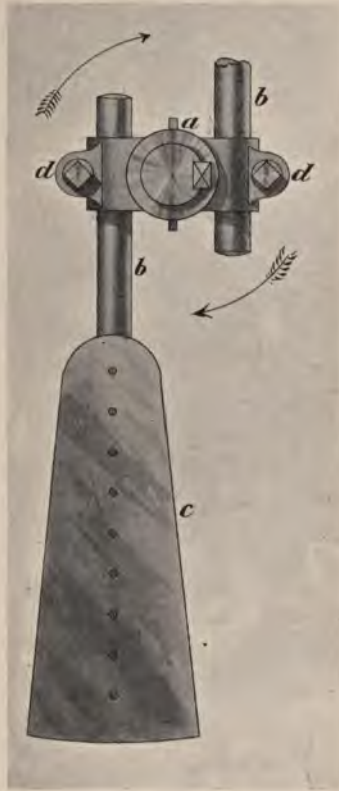
Fig. 17.—The hub and one of the blades of the screw on the Farman machine. The blade c , is a sheet of metal riveted to the rod b , and forms a projection on the back of the blade which greatly reduces its efficiency. The peculiar form of hub employed makes it possible to change the diameter and pitch of this screw at will.
